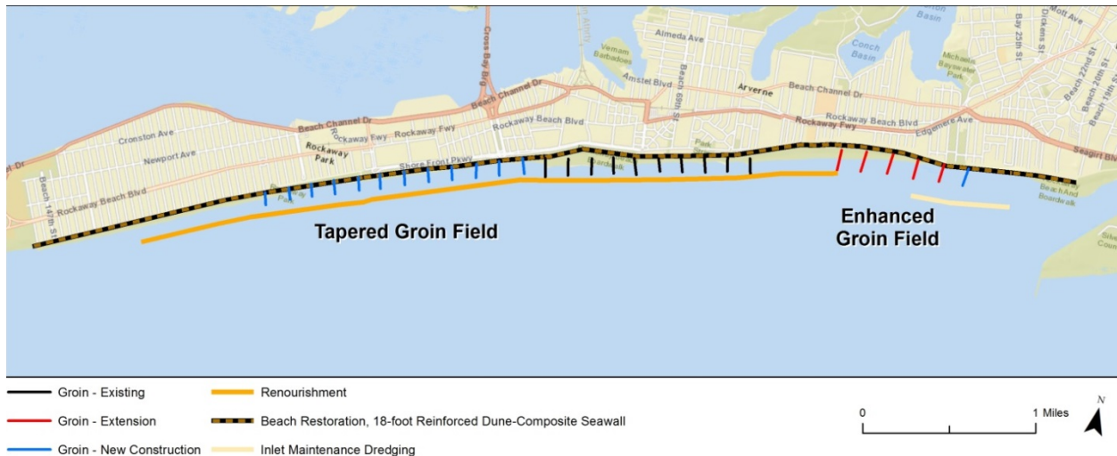
Figure 5-4: Beach Restoration with Beachfill, Groin Extensions, and New Groins
